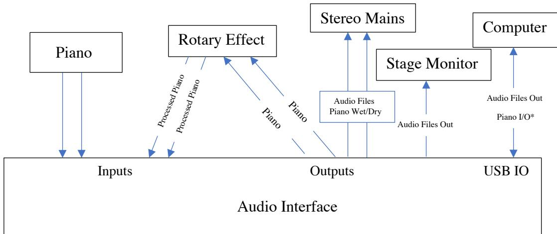
\*The diagram above illustrates that the piano signal may be sent to and from the computer. This is in case the rotary effect and reverb are added using VSTs.
